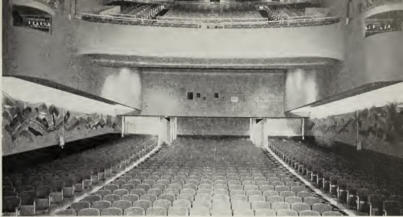
The old auditorium, above, presented a remodeling problem because of the boxes from the balcony to the proscenium on each side. A projecting structure over wall aisles, made of plaster on metal lath, right, solved the problem well.
